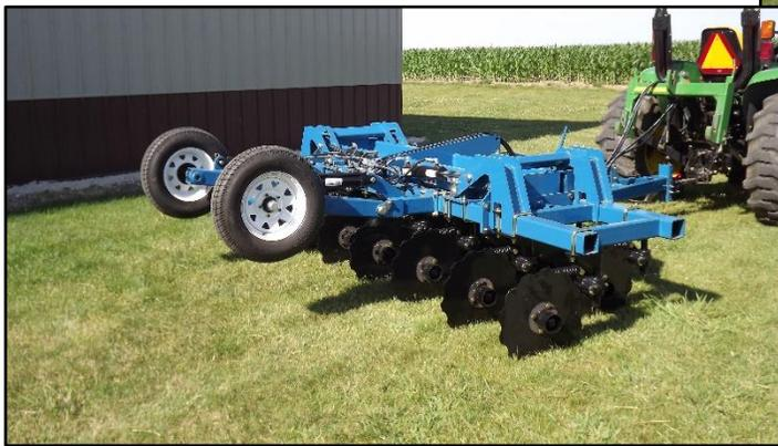
The Solaris SCX Straw Crimper's discs can pivot left and right and up and down independently, leaving a well-secured, even mulch installation
