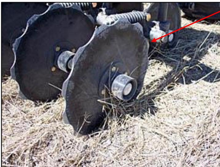
When an SCX crimper disc hits an object, it floats over or pivots around it, while the other discs remain firmly engaged with the soil. The disc pivoting action also allows for smoother, tighter turns for faster installation.
